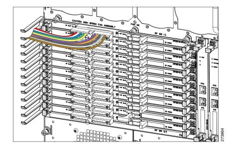
**Step 5** Repeat steps 1 through 4 for the remaining 11 UCH to RF switch card interconnects.
